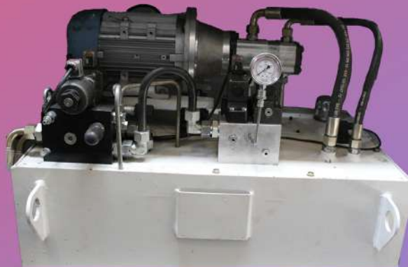
DUAL PUMP SYSTEM
