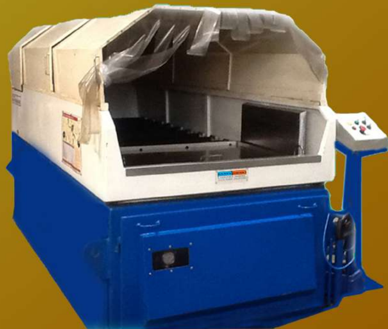
OPEN TYPE PRESSURE CLEANING MACHINE WITH ALKALINE WATER WITH 60°C TEMP AND 140 bar Pr
