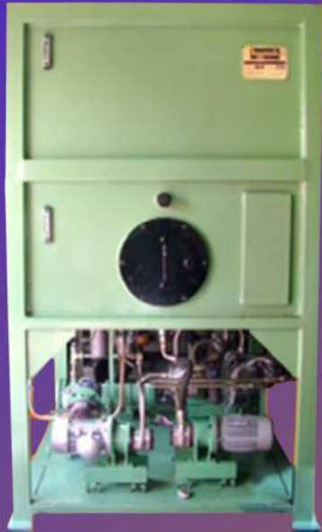
TRANSFORMER OIL CHAMBER TEST RIG
