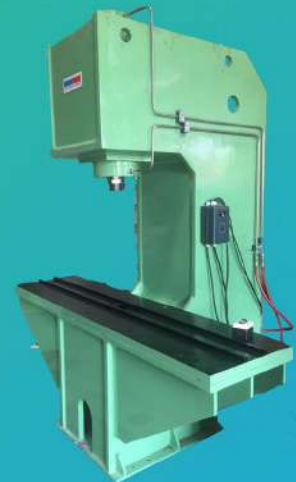
40 TON BEND REMOVING
